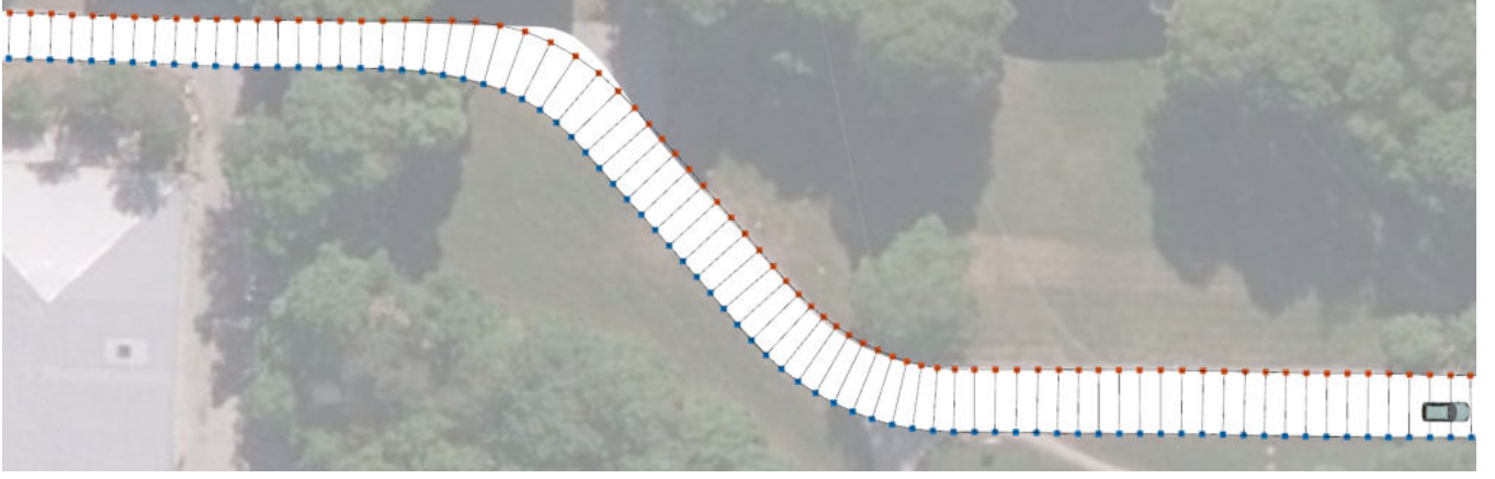
Fig. 11: Right (blue) and left (red) lane boundaries of our road estimate in comparison with the ground truth from an HD map (white).
